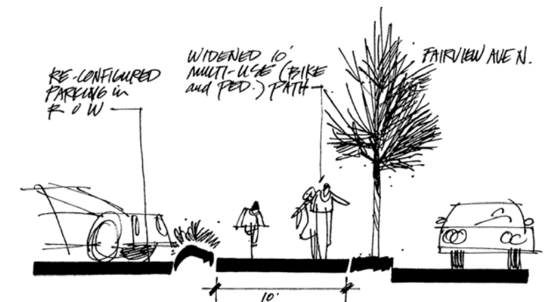
Cross-section of new widened path along City Light right-of-way on Fairview Avenue North.
